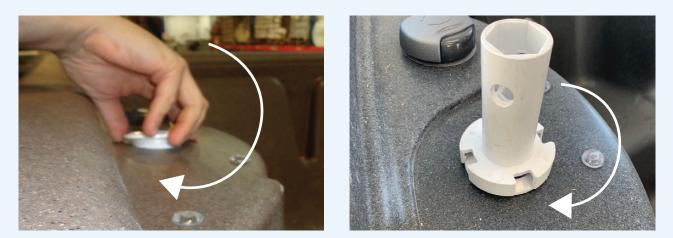
**10** Screw on the faceplate and keep one hand on the jet underneath to prevent it from moving. Tighten with the wrench tool and reinstall the top of the waterfall.
