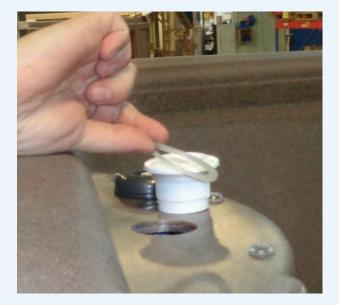
6 Once unscrewed, please be careful to keep the flat gasket that is between the jet and the spa wall. You can reuse or replace it with the new one that will be sent to you;
