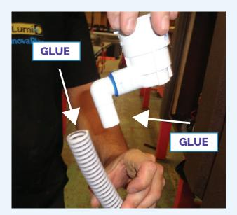
8 Put glue on the 90° adaptor and in the top of the inner pipe. Then, insert the 90° adaptor as deep as possible in the pipe;
