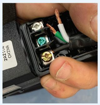
3 3- Place one wire at a time in its position, according to the color.
