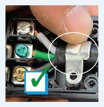
5 Add the metal plate and screw. Make sure to put it on the right side as above:
