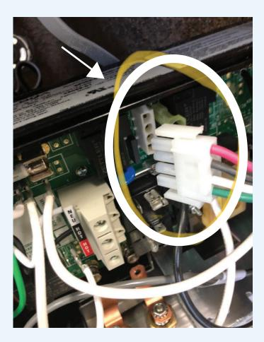
A Remove the connector plugged into the circuit board and finger-tighten the tabs on either side of the white end cap to remove it easily (pump connection);
